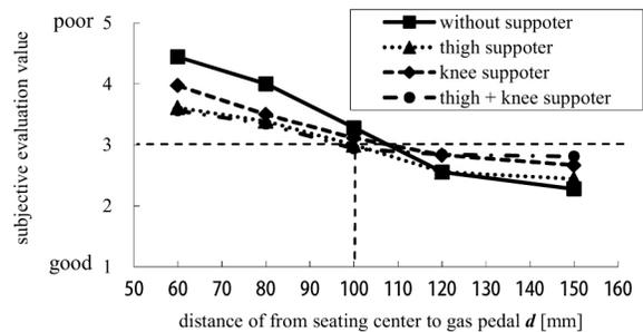
Figure 9. The relationship between subjective evaluation rating and  $d$  in each supporter's condition
