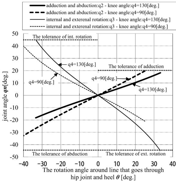
Figure 13. Each joint's rotation angle according to the two seating height
