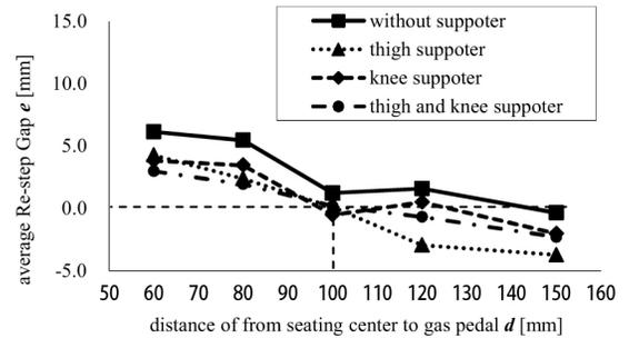
Figure 8. The relationship between  $e$  and  $d$  in each supporter's condition
