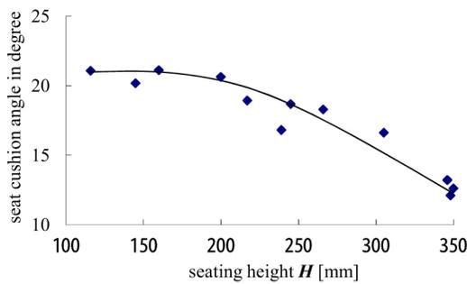
Figure 10. The relationship between seat cushion angle and H for passenger cars in stock
