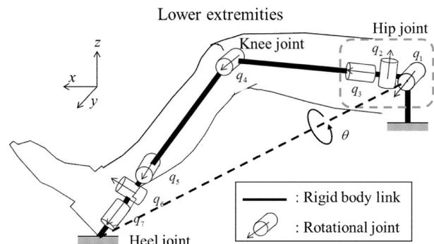
Figure 12. The rigid link model for computation
