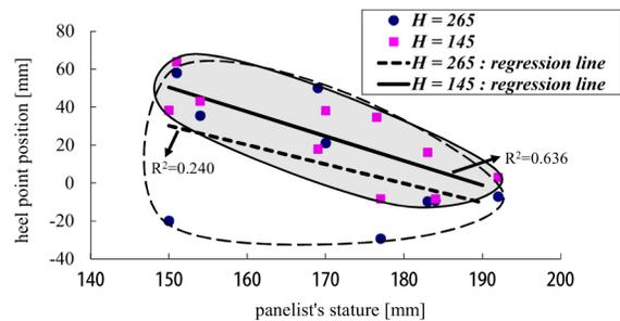
Figure 14. The relationship between stature and heel position for the two seating height
