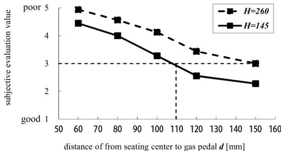
Figure 7. The relationship between subjective evaluation rating and  $d$  in the two seating height
