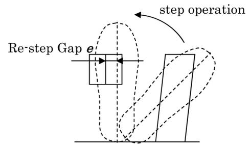
Figure 3. The definition of the re-stepped gap  $e$
