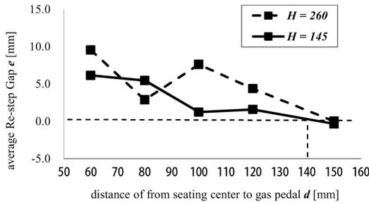
Figure 6. The relationship between  $e$  and  $d$  in the two seating height
