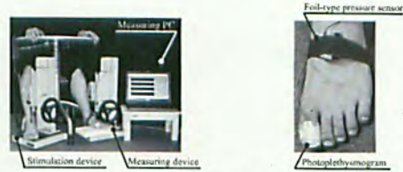
(a) Experimental apparatus for measuring pulse waves of dorsalis pedis artery (b) A close-up view of measuring devices
