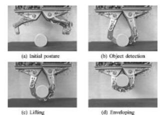
Fig. 10. Sliding-based grasp.
