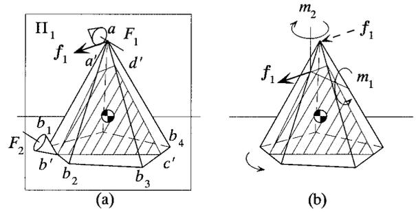
Fig. 4  $f_1$  at  $a$  produces  $f_1$  and two moment components at  $a'$
