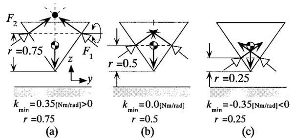
Fig. 7 Explanation of gravitationally stable equilibrium
