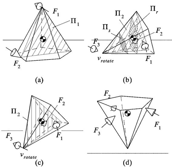
Fig. 9 A procedure for a general polyhedral cone object
