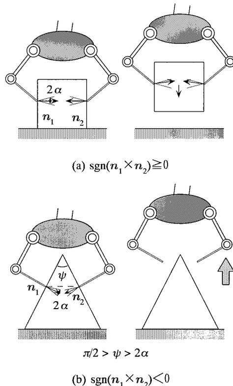
Fig. 1 Two examples of direct grasp
