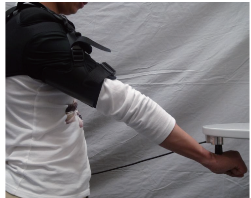
Figure 8. Experimental condition: the subjects exert force on the force sensor
