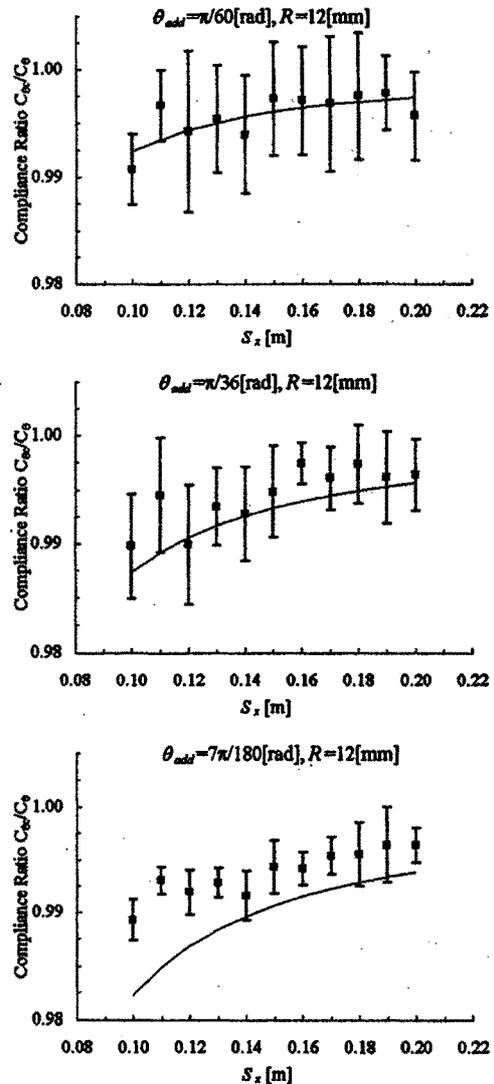
Fig.7 Experimental results of compliance ratio between an edged and a curved objects.
