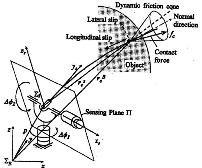
Fig.1 An example of 3D Active Antenna
