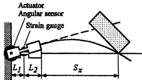
Fig.6 Sensor geometry of the experimental system
