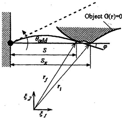
Fig.2 A 2D Active Antenna contacting an environment
